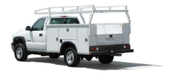
Pictured above is a 98" Long Utility Body 40" High with Vertical Door Arrangement and Open Top Compartments and Optional Over-Cab Rack on a 56" C.A. Single Rear Wheel Truck. Standard features include open top lids covered with aluminum diamond plate, stainless steel tailgate guard and heavy-duty Class III recessed rear bumper. For 3/4 ton and 1-ton trucks with single rear wheels - 56" Cab to Axle.
